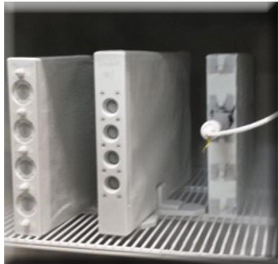
Plastic with accumulated total 90 days @ +55°C and 90% relative humidity with multiple exposure cycles @ -30°C
